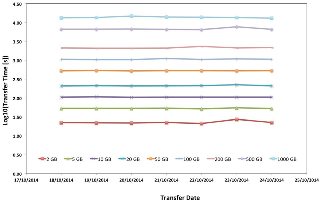
Figure 2. Daily data transfer speeds between the NCI and the University of Melbourne. There is little variability in the transfer times during the week for each of the file sizes.
