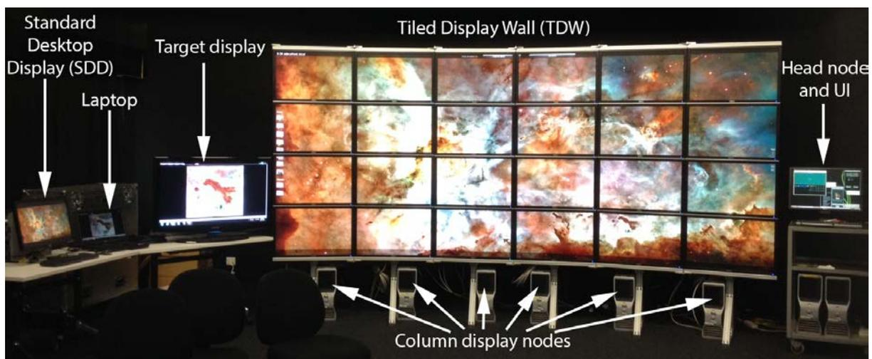
Figure 1. Configuration of the OziPortal tiled display wall used by Meade et al. (2014). The six columns and four rows of Dell UltraSharp displays (2560 x 1600 pixels each) combine to produce a 98.3 Megapixel image (15360 x 6400 pixels). Note the presence of bezels between pairs of displays, which can distract from the visual content. The displayed image is the Carina nebula (image source: <http://hubblesite.org/gallery/album/nebula/pr2007016a/hires/true/>).
